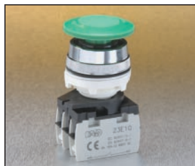
T11ED02-C maintained, 40mm diameter mushroom head, green with clip and two contacts
