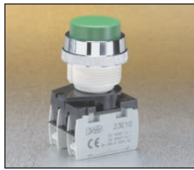
T11CB02-C maintained, round, projected, green pushbutton with clip and two contacts
