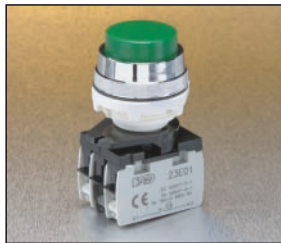
T11AK20-CL120 momentary, round, projected, green pushbutton with clip, two contacts, lamp block and 120V LED bulb
